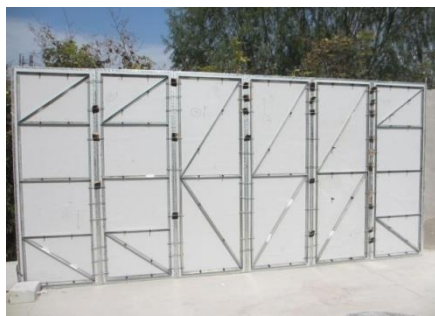
Figure 3. Group 2 supported formwork
