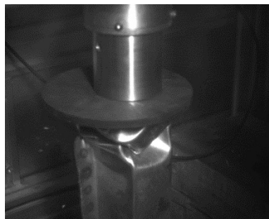
Figure 4. Deformation of the test piece.
