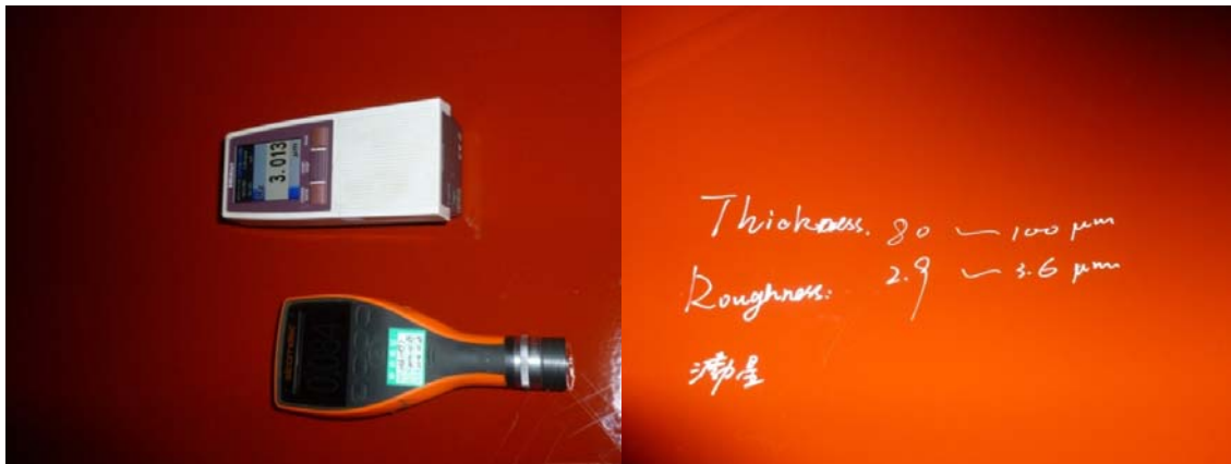
Figure 2. Test record of dry film thickness and roughness
