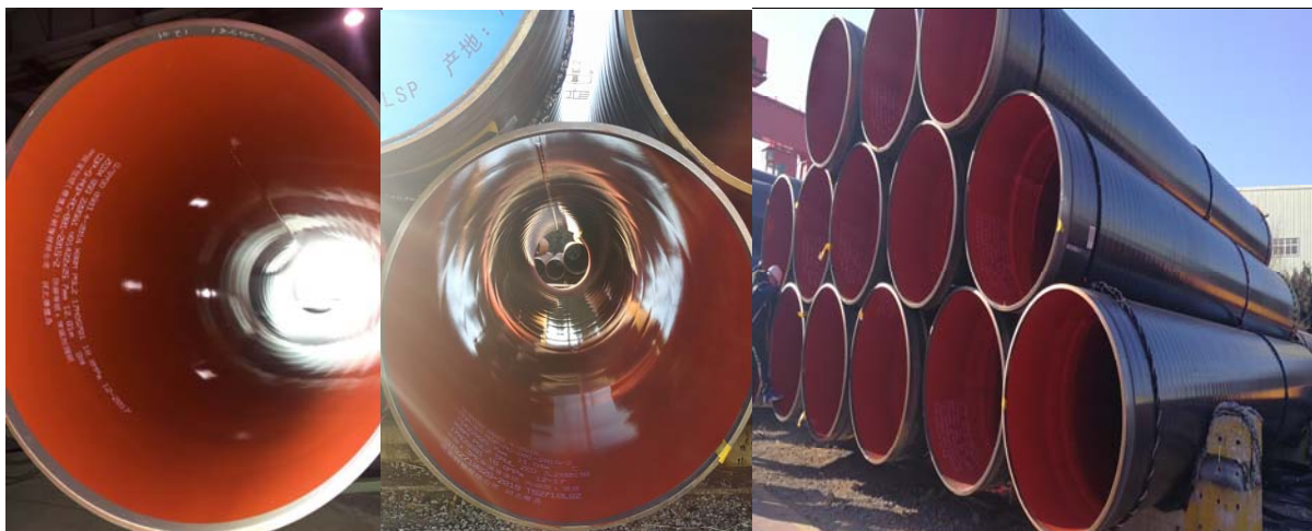
Figure 1. Pipeline of after spraying solvent-free epoxy internal drag reducing coating
