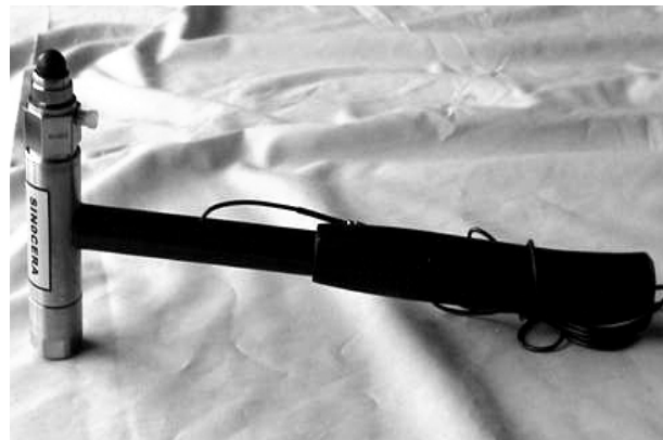
Figure 1. CL-YD-305A force hammer
