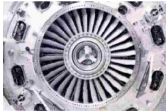
Figure 3. Engine blade of TiAl based alloy.
