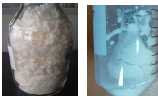
Figure 2. Encapsulated Lactobacillus acidophilus by freeze-drying (left) and by spray-drying (right).
