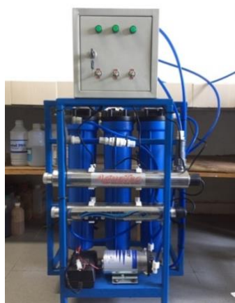
Figure 2. UV-Ozone Wastewater Instrument
