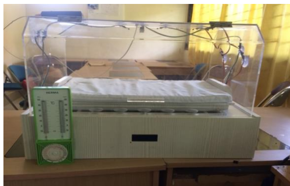
Figure 4. Design of the incubator box complete with the sensor.
