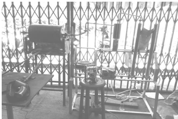
Figure 2. The snapshot of waste tire pyrolysis apparatus.
