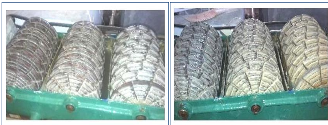
Figure 3. Biofilm formation in RBC, (a) at the end of acclimatization, (b) at running processing system
