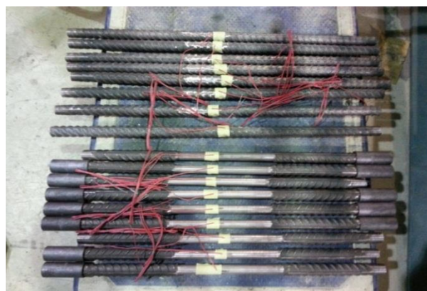
Figure 1. Fuse bar equipped with strain gauges
