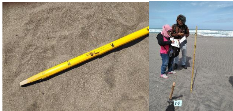
Figure 6. The damaged staff number 2 (left) and replacement for the missing staff number 14 (right)
