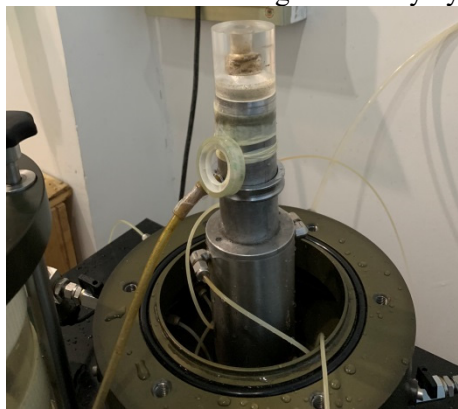
Figure 3. The plastic plug over the split mould.
