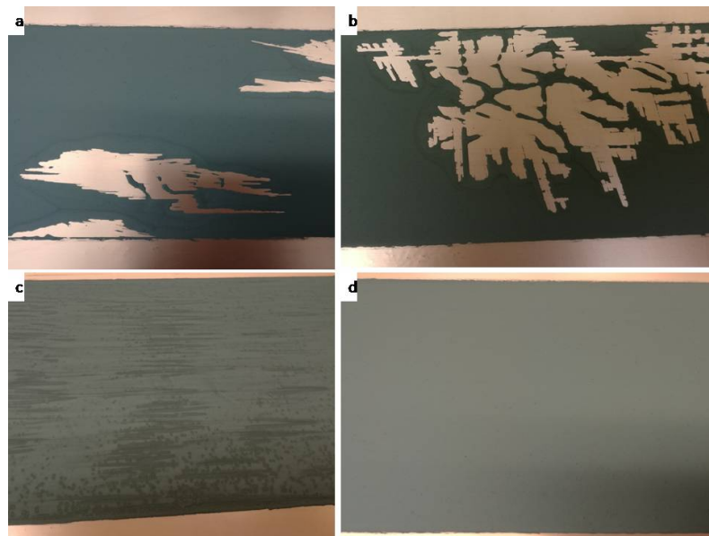
Figure 1. The photos of the anodes plates: a: the "SiO/C is 5/95" anode using water as solvent during slurry. b: the "SiO/C is 20/80" anode using water as solvent during slurry. c: the "100% Graphite" anode using water as solvent during slurry. d: the "SiO/C is 20/80" anode using 10 % isopropyl alcohol solution as solvent during slurry.
