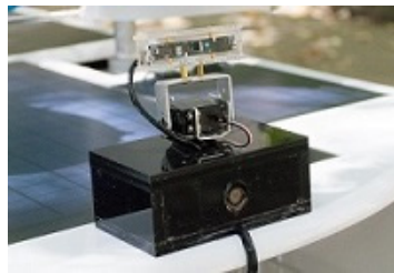
(a) Installation of camera head and pan/tilt.
