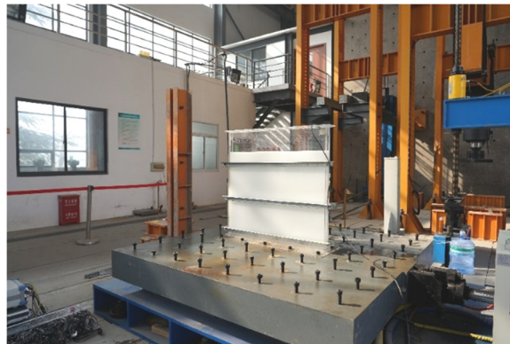
Figure 3. Rectangular tank model structure and shaking table
