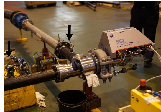
Figure 5. Test and pressure port location overview, 2 ID upstream, 6 ID Downstream.
