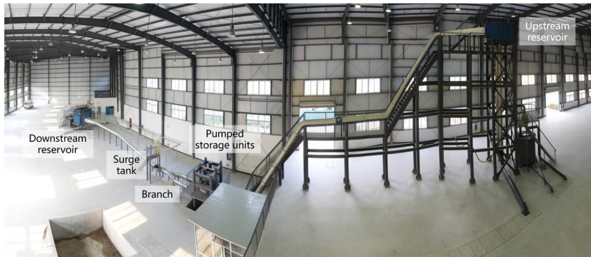
Figure 1. Photo of the experiment platform for transient processes of pumped storage plants.
