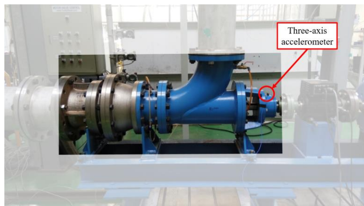
Figure 3. Mixed-flow pump and accelerometer location.
