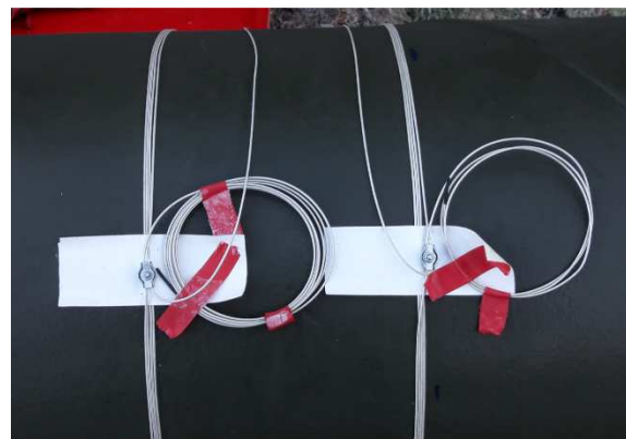
Figure 6. Mounting example - 4 turns on 0.45 m diameter pipe.
