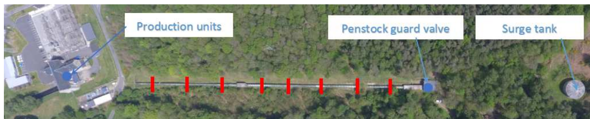
Figure 8. Pressure measurement scheme - classical sensors (blue) and PVDF wires (red).
