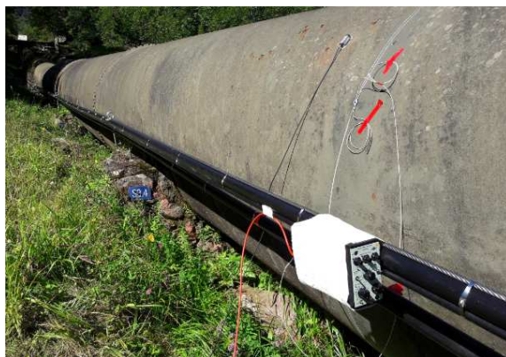
Figure 5. Mounting example - 1 turn on 1 m diameter pipe - wire and amplifier.
