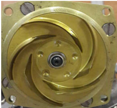
Figure 1. Impeller without any balancing hole.
