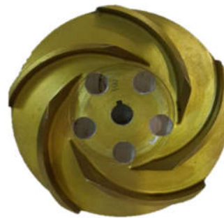
Figure 2. Impeller with balancing hole.
