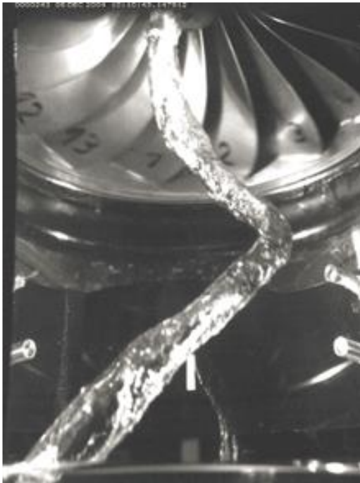
Figure 1. Vortex rope visualization for the part load operation of Francis turbine [1].
