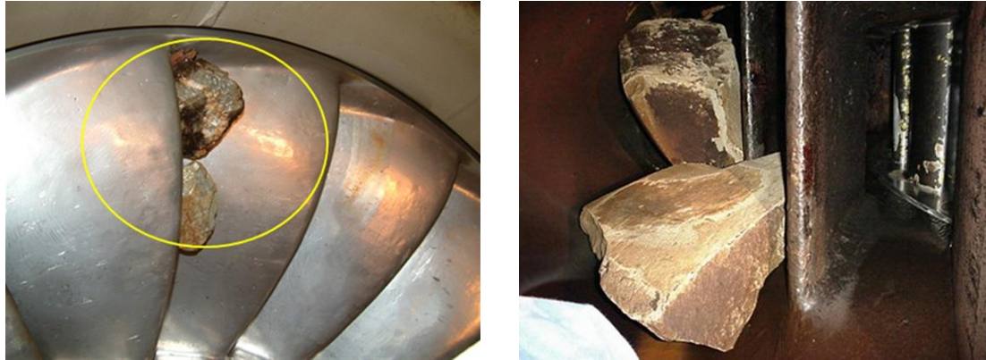
Figure 1. Typical blockage on a turbine runner (left) or distributor (right) [6].
