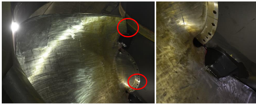
Figure 1. Prototype. Two stop blocks on the pressure side of the blades to fix the opening.
