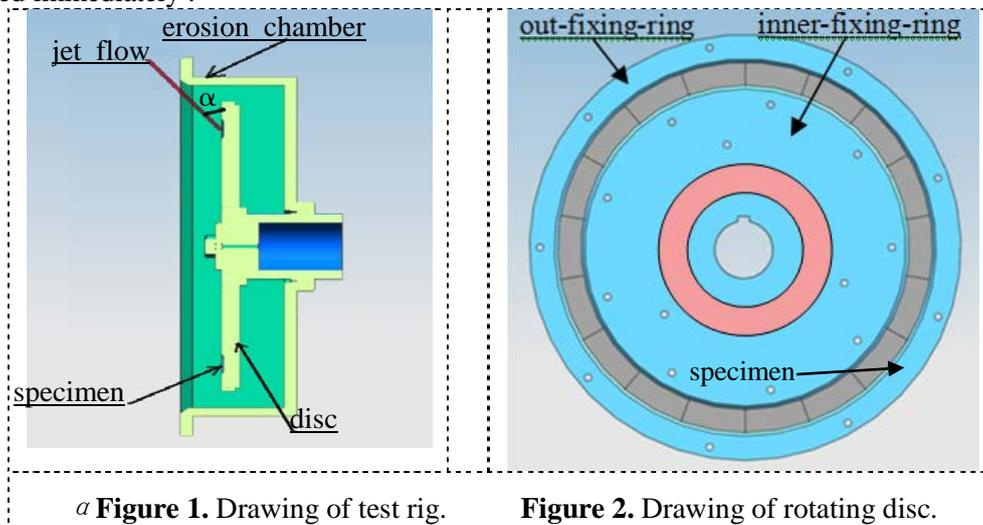
*a* Figure 1. Drawing of test rig.
