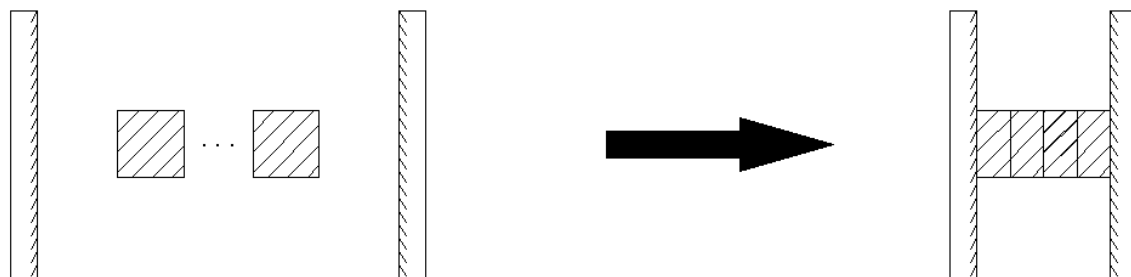
Figure 2. Gluing process of Wheat Straw Particleboard (urea formaldehyde adhesive)
