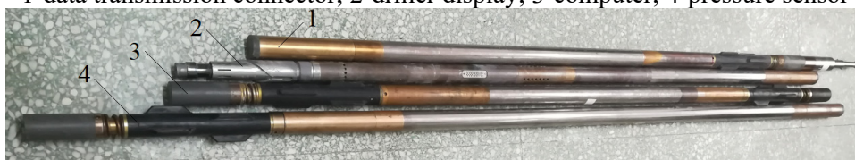
Figure 7. Downhole instrument of TD-MWD1 wireless MWD measurement system 1-master control; 2-pulse signal generator; 3-inclinometer probe; 4-battery
