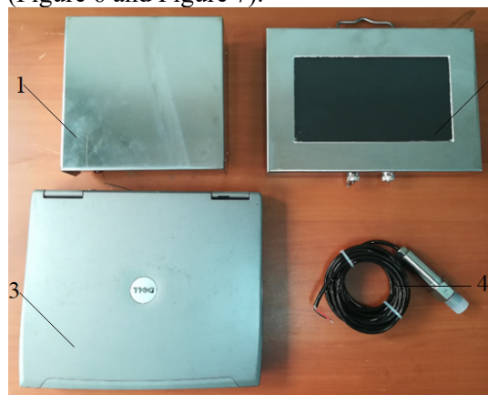
Figure 6. Ground equipment of TD-MWD1 wireless MWD measurement system 1-data transmission connector; 2-driller display; 3-computer; 4-pressure sensor
