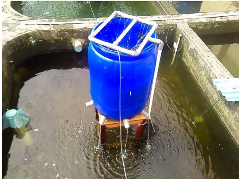
Figure 2. The implementation of trickling filter on the fish pond
