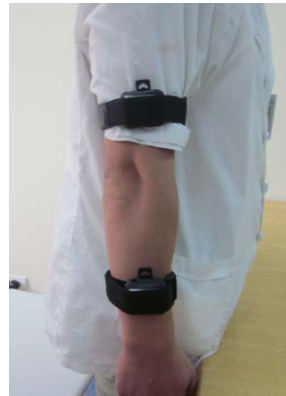
Figure 2: Fixed position of the 9-axis wearable sensor nodes
