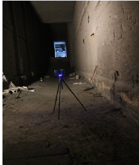
Figure 4. Mapping the internal structure parameters of flue using the 3D laser scanner.
