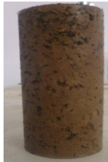
Fig.2 Waste tire particle reinforced lime-ash soil sample
