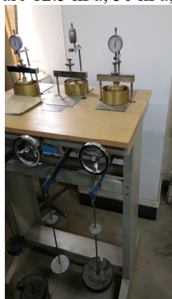
Fig.3 Standard compression test
