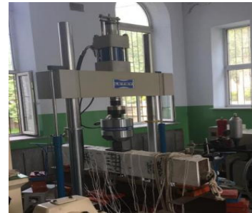
Figure 3 PA-100 Electro-hydraulic Servo-based Dynamic and Static Fatigue Testing Machine
