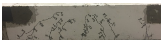
Figure 9 Image of Cracks on Test Beam P4 Due to Fatigue Loading
