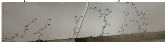
Figure 4 Image of Cracks on Test Piece P1
