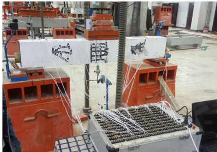
Figure 2 Hydraulic Jack-based Static Force Loading Device
