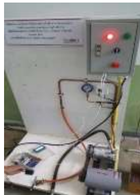
Figure 6. The in-house flammable gas detection system tested its function with the biogas filler.
