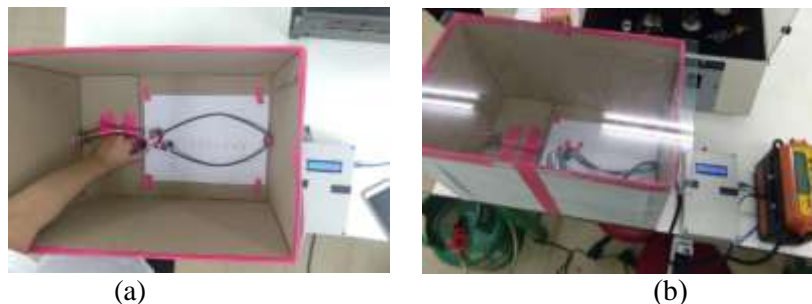
Figure 4. Butane investigation (a) and biogas investigation (b) with the flammable gas detecting system setup.
