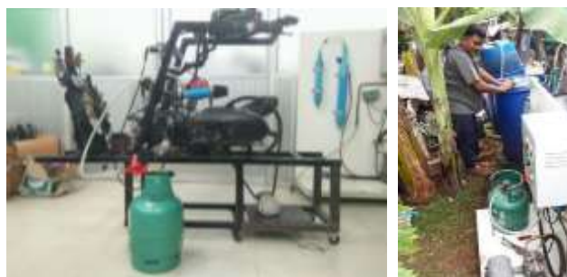
Figure 2. The biogas filler (Left) from Jettarach [9] and the hybrid engine (Right) from Pramuanjaroenkij et al. [10] which was used to investigate generator transmission systems.
