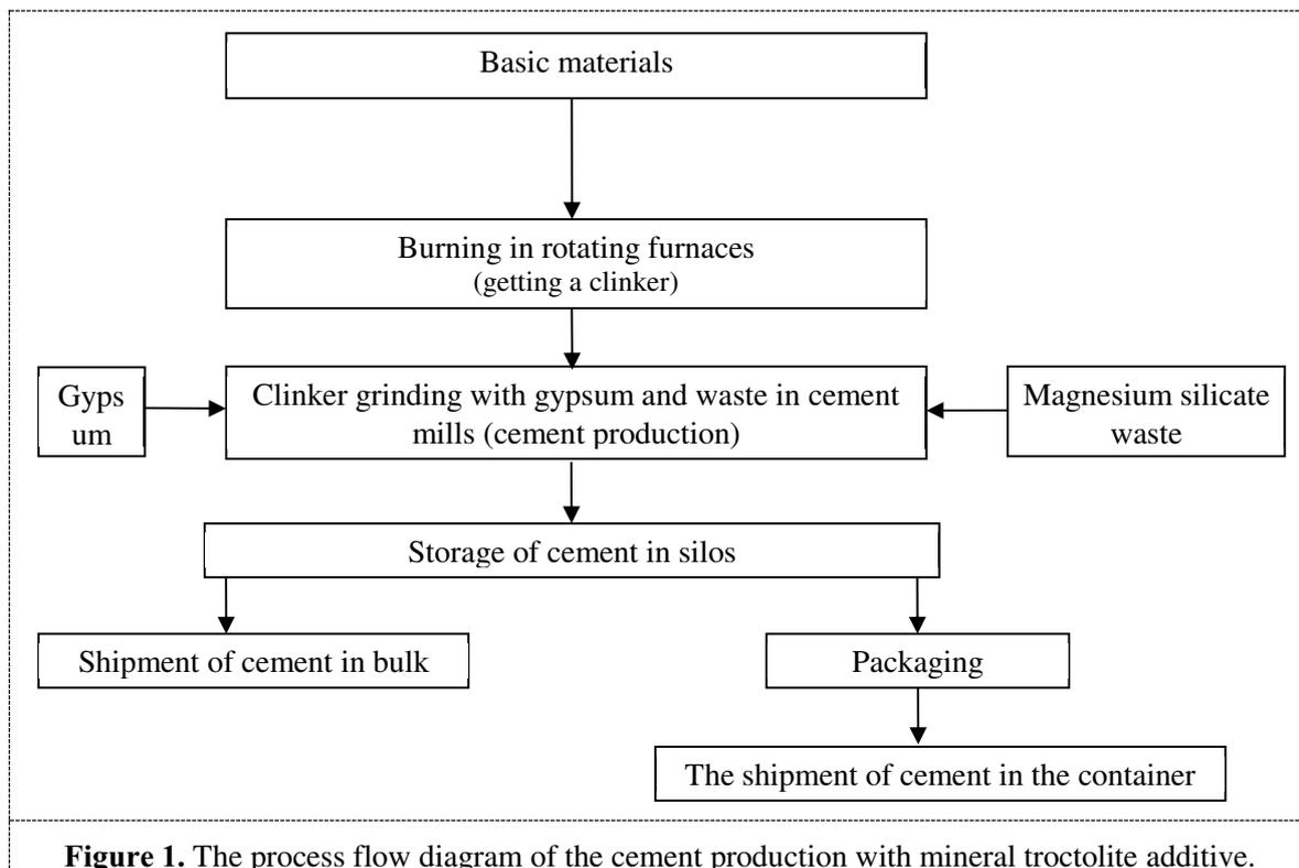
The production of cement with mineral additives excludes the introduction troctolite in the raw material mixture for burning that positively effects on the cost of cement and influence on the environment.
