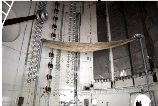
Figure 11. DC voltage flashover test layout.
