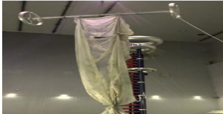
Figure 6. DC voltage generator and test layout.
