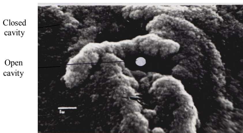
Figure 2. The surface of the chips in chipboard coated with the cured binder with a view to the not destroyed vapor-gas bubbles in the binder.
