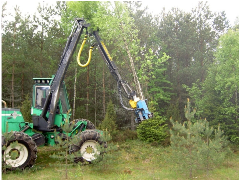
Figure 1. Harvesting thin trees with the help of the multiple-tree accumulating head (photo by the author).
