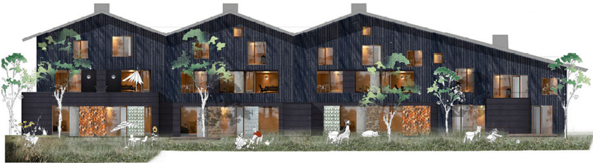
Figure 10. Visualization showing reused materials that embellish the ground floor façade. The project has single story flats below and terraced housing above.
