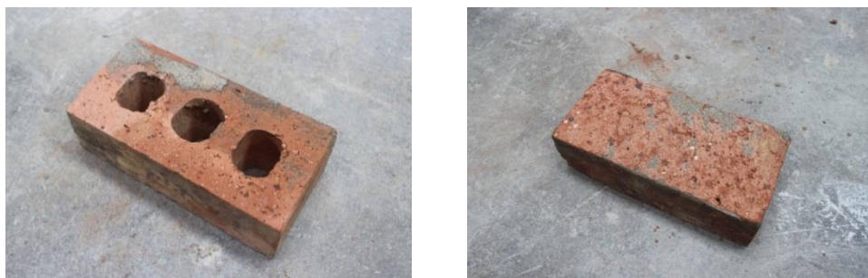
Figure 4 (a). Reclaimed bricks by saw-cutting method.
