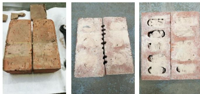
Figure 4 (b). Reclaimed bricks by punching method.
