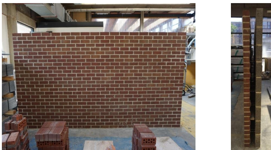
Figure 5. Full-scale masonry wall.
