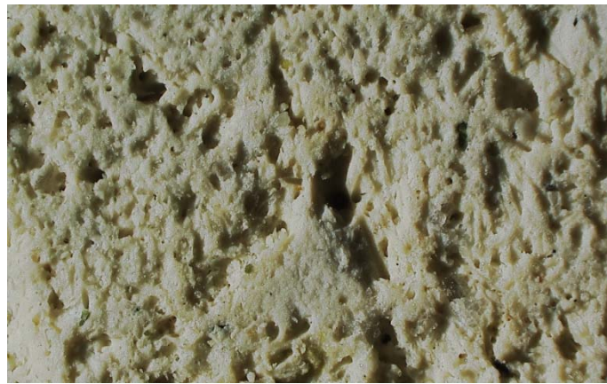
Figure 1. Opoka-rock - Porous texture -Digital microscopy (Photo. A. Pękala)
