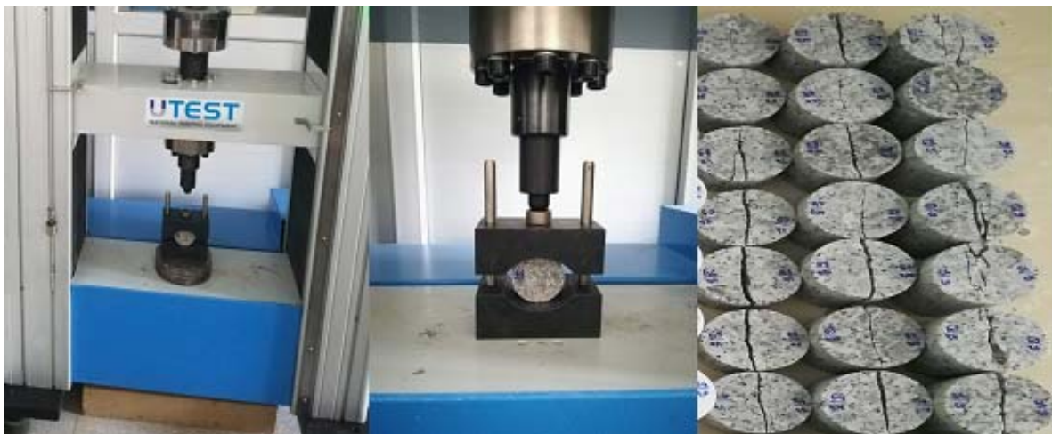
Figure 1. Brazilian test samples in different t/d ratios.
