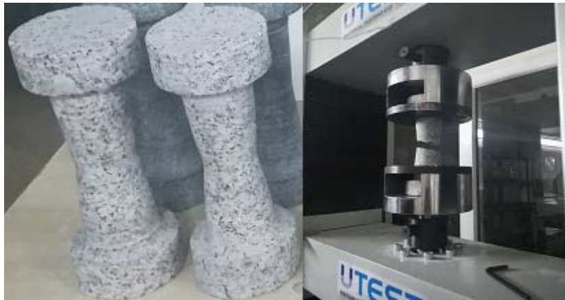
Figure 2. Dumbbell shape specimens for direct tensile test and electromechanical universal test machine
