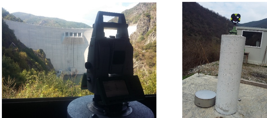
Figure 5. Measuring setup- acquisition of laser scan data for accurate change detection
