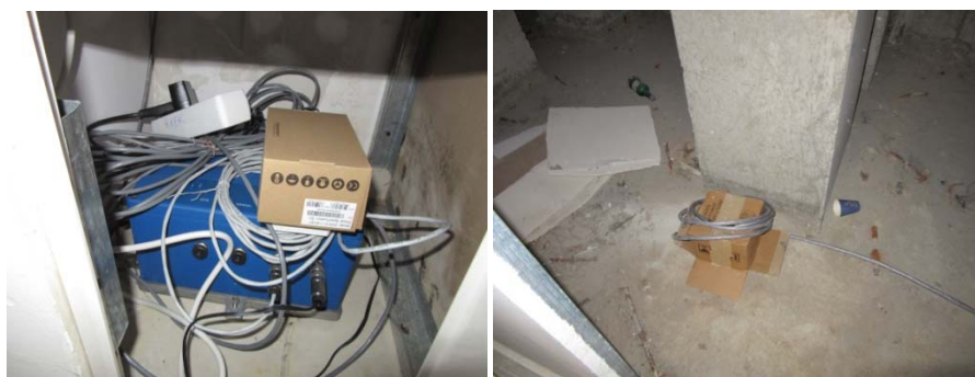
Figure 1.c) GMS18 GeoSIG station at the ground floor (left side) has been replaced with a triaxial sensor connected directly at the Granite multichannel station
