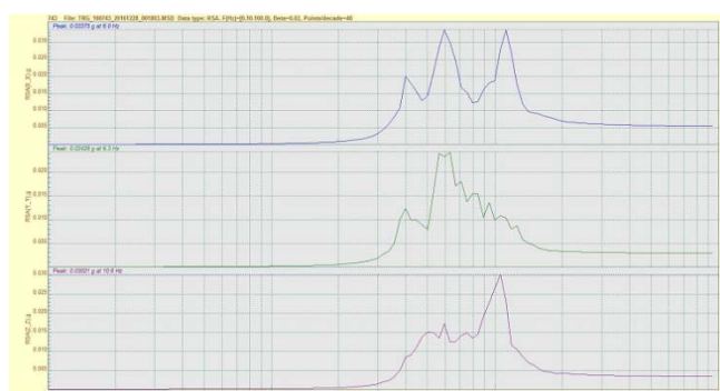
Figure 4. Acceleration Response Spectrum for X, Y and Z directions. Tripartite representation of acceleration, velocity and displacement spectra (channel 7)
