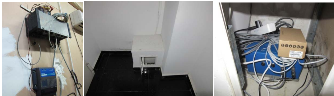
Figure 1.b) The GRANITE station installed with 3 sensors (at the top level, level 4 and basement) and a GMS18 GeoSIG station at the ground floor (which it will be removed further – figure 1.c)
