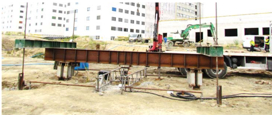
Figure 6. The view of CFA in situ load tests
