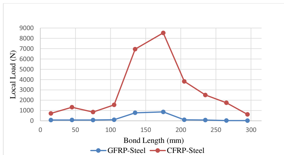
Figure 7: Comparison of Local Load between GFRP-Steel and CFRP-Steel at 12 kN Applied Load
