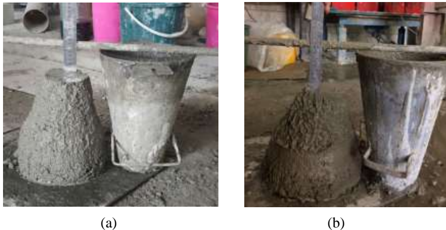
Figure 3. Types of slump for (a) CONC mix and (b) EMC mix.
