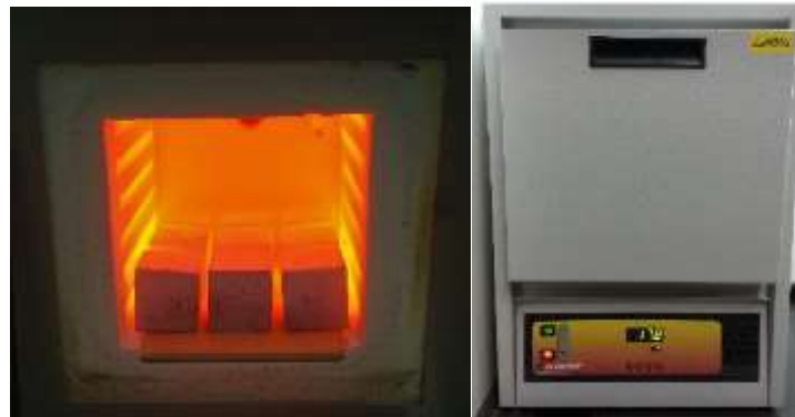
Figure 2. Set-up for heating of specimens.
