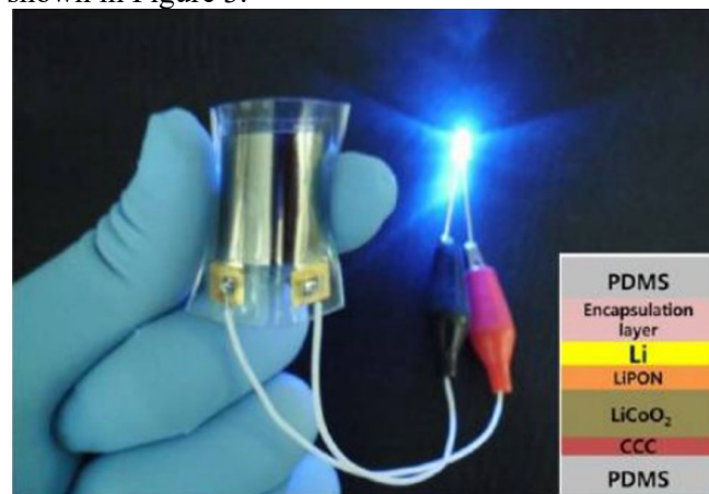
Figure 3. Schematic diagram and picture of flexible LED system integrated with Flexible TFLBs [89]
