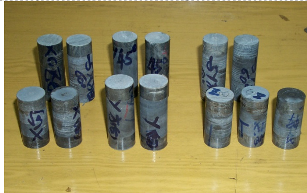
Figure 2. Acoustic emission testing of rock core objects
