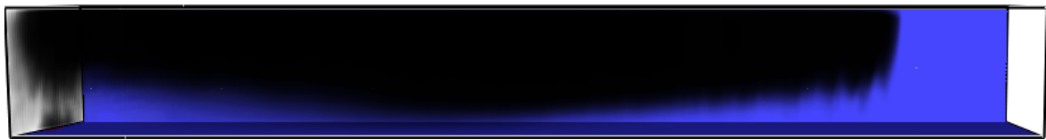
(a) The movement of smoke at the end of the simulation when the air curtain is in the position of 5m in tunnel
